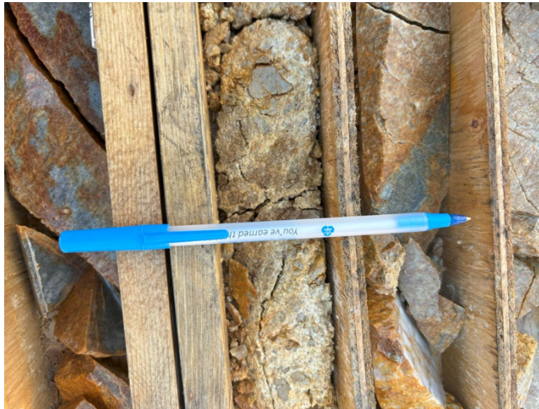
Figure 12.6 Supremo Deposit Drill Core – Brecciated Granodiorite
