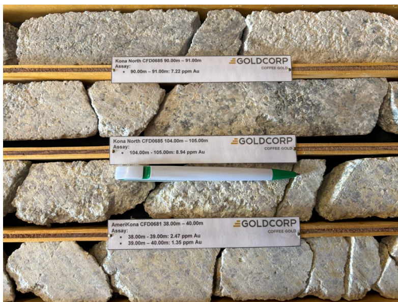
Figure 12.8 Kona Deposit Drill Core – Subtle Brecciation
