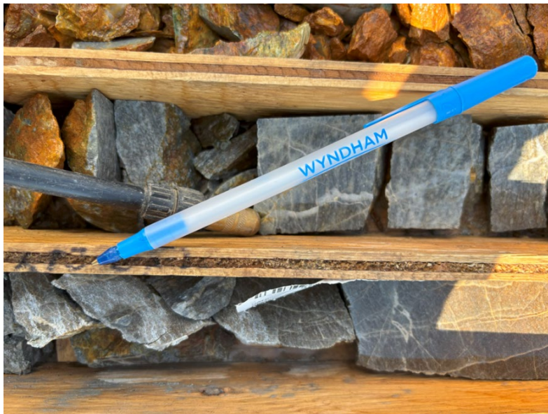
Figure 12.7 Latte Deposit Drill Core – Biotite Schist with Silicification
