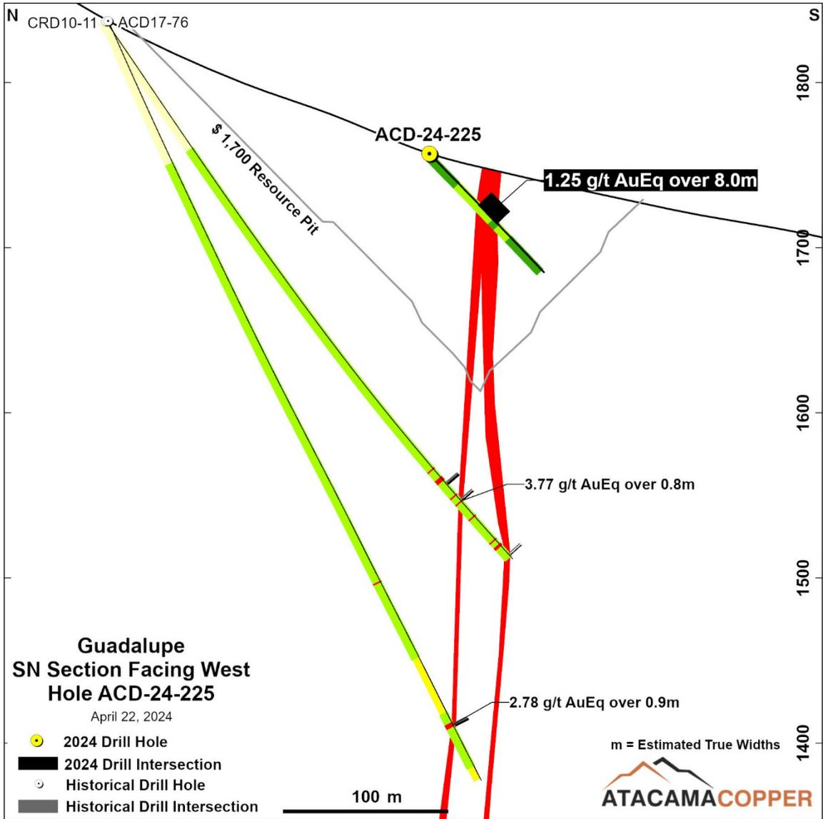
Figure 6 – Cross-section through the Guadalupe vein system with hole ACD24-225
