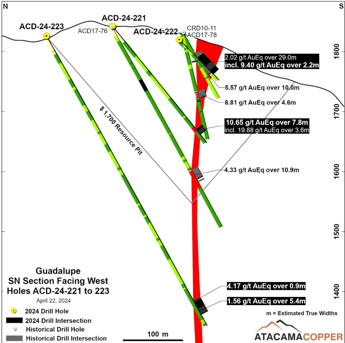
Figure 4 – Cross-section through the Guadalupe vein system with holes ACD24-221, -222 and -223
